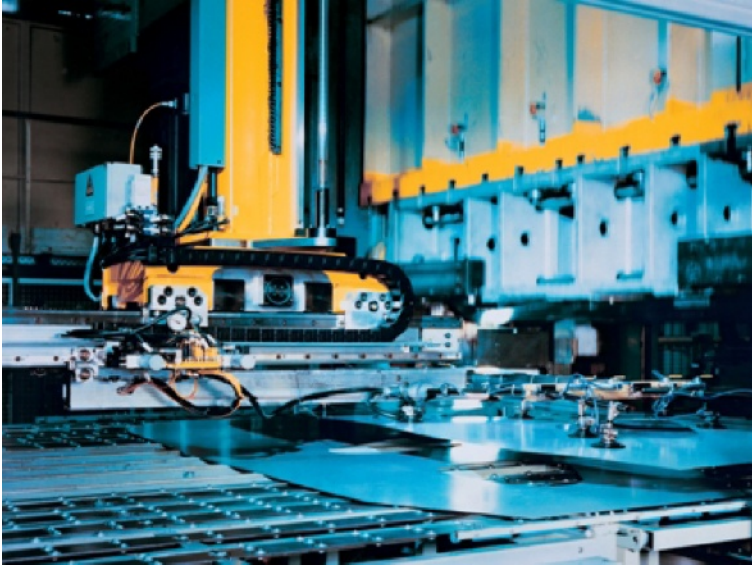
Fig. 1.1 Example industrial system. Press transfer system in sheet-metal working. Courtesy of Bosch Rexroth AG
